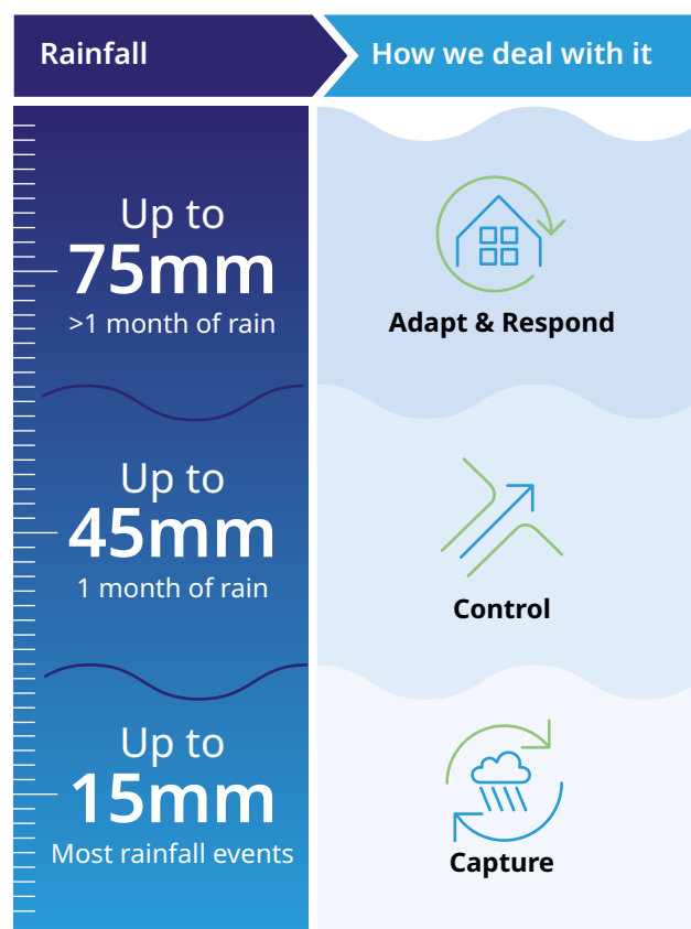
Figure 3: Our flexible approach to surface water management
